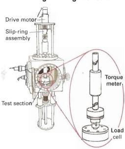
At Glenn Research Center, Cleveland, Nye and NASA have compared MAC and PFPE performance in oscillating bearing test rigs.
