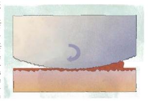
rupture can result in high wear, high temperature, and premature heat aging of the elastomers of seals.
